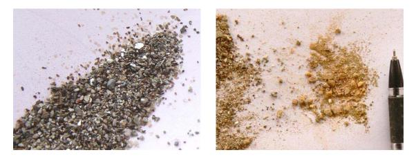
Similar as in the mountain areas, the tested soils are too fine to be utilized for compressed stabilized soil blocks. Also these samples contained a lot of soft stone particles, which may have a negative effect on the compression strength of the blocks. The right picture shows an example from Lekhnath Chowk, where the particles that look like gravel can easily be grinded to powder between the fingers.
