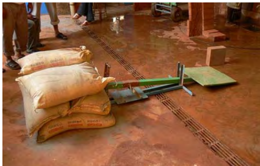
Testing the strength of the blocks by a home-made bending test.
