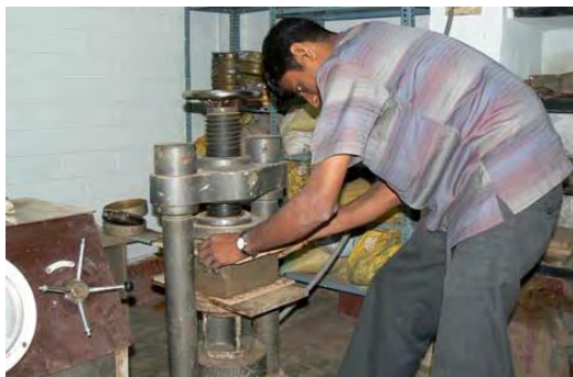
Testing the strength of blocks with the compressing machine.
