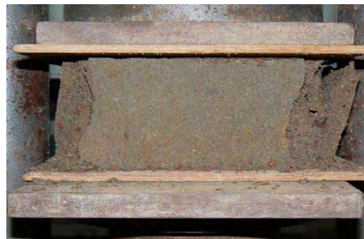
Testing the strength of blocks with the compressing machine.
