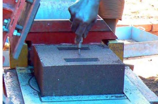
Test the compression of freshly made blocks with the penetrometer.
